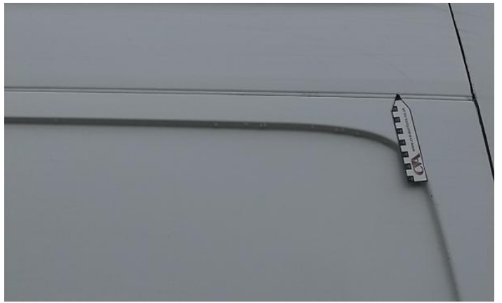
10: Door nsr Dented With Paint Damage
