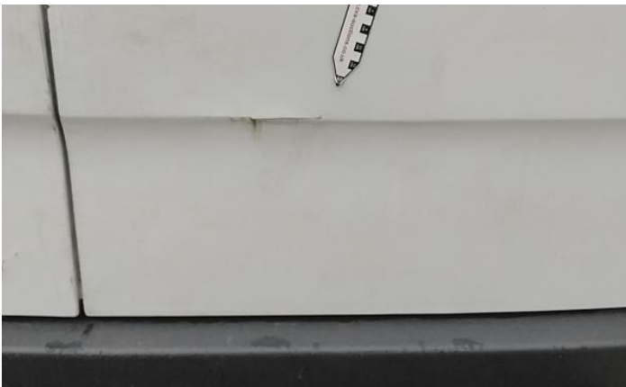
17: Door nsr Dented With Paint Damage
