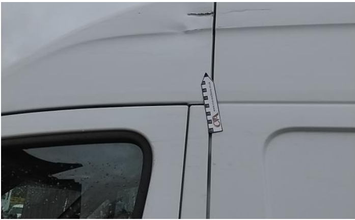
9: Door Moulding nsr Scuffed (Unpainted) Over 100mm
