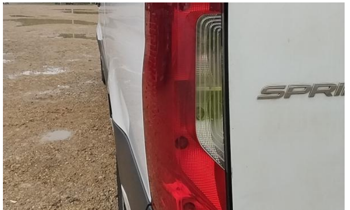
18: Door osr Dented With Paint Damage
