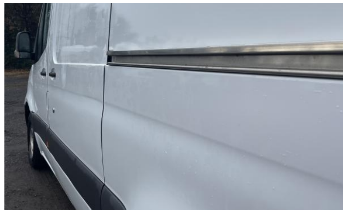
3: Qtr Panel osr Poor Previous Repair Rippled UpTo 30%
